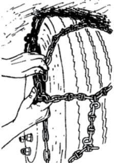
Tighten with the tightening cam by inserting a tightening lever into the groove of the cam and twisting it 90 degrees so that the chain loop slips into the locked position (6).
