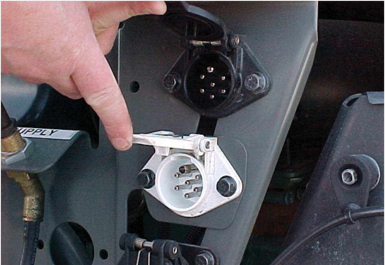
The top socket is the 24N with the solid top pin and the one below is the 24S with the hollow top pin.
