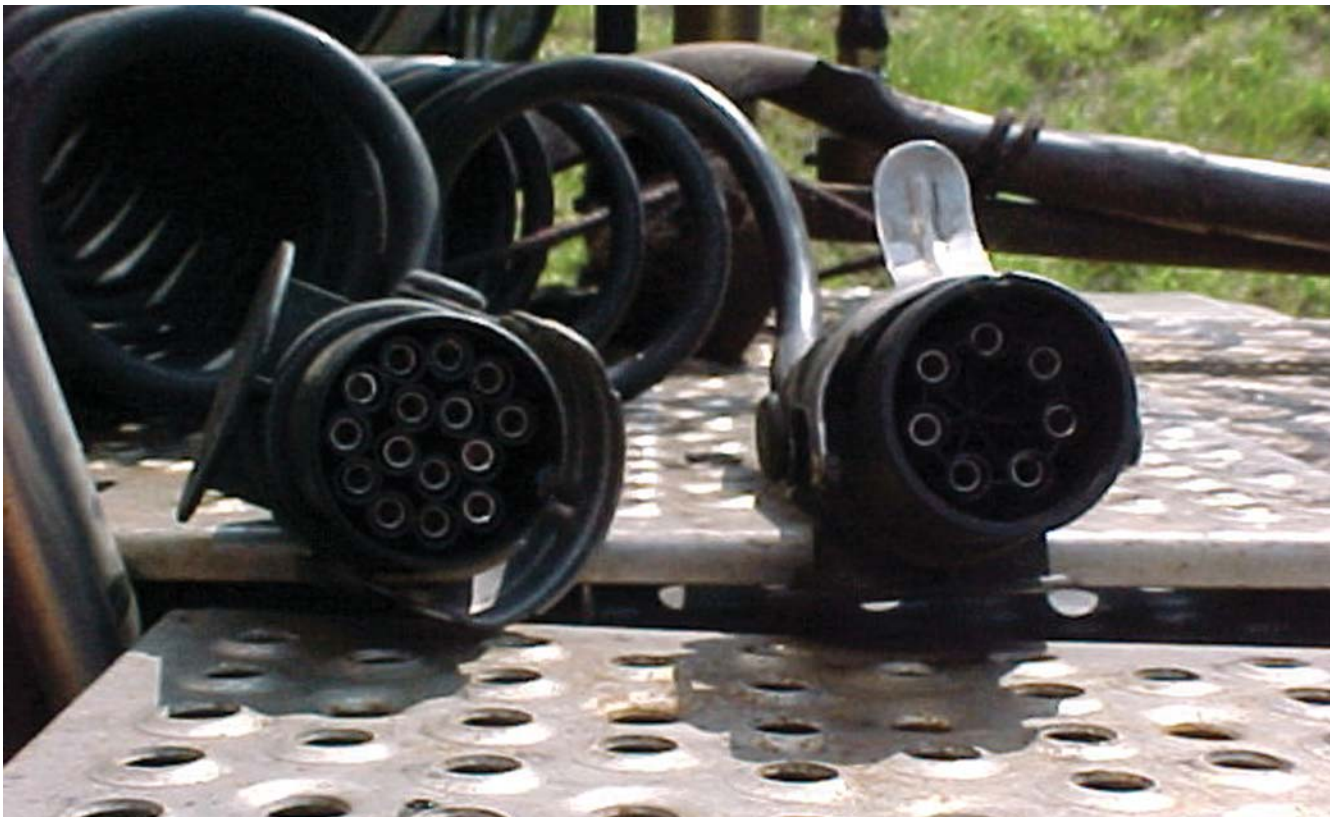
Left hand side 15 pin continental lighting plug ISO 12098, on the right 7 pin ISO7638.
